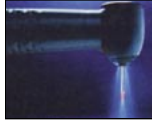
Figure 1. The beam is focused approximately 1.5 mm from the fiber tip. The red color is the aiming beam. The 2780 nm wavelength is invisible to the human eye. Note how the column diverges as the distance from the tip increases.
